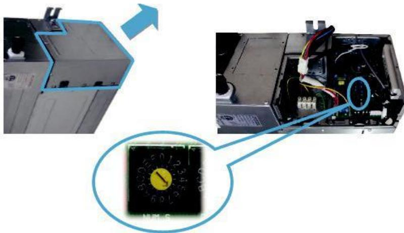
Select one of positions to set suitable static pressure according to the instruction sticker on the back of the cover of electrical box.
